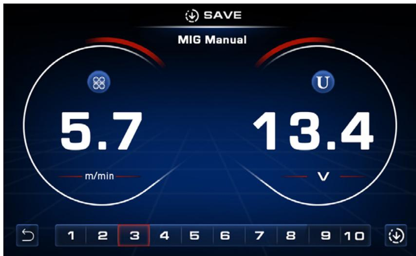
You can reach the Save Jobs menu and Load Jobs menu from any of the welding screens. Press and hold the **Left Action Button** to reach the Save Jobs menu, press and hold the **Right Action Button** to reach the Load Jobs menu.
