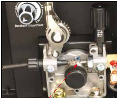
(5) Feed the wire through the drive roller and into the outlet guide tube of the wire feeder. NOTE: MIG 165 not geared
