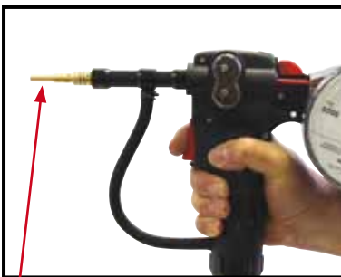
(11) Fit the contact tip over the wire and screw it into the tip holder, nip it up tight.
