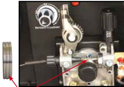
(11) Install a U groove drive roller of the correct size for the diameter wire being used. NOTE: MIG 165 not geared
