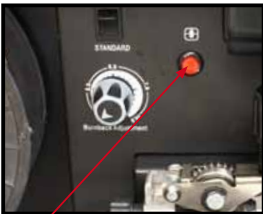
(9) Close down the top roller bracket and clip the pressure arm into place. NOTE: MIG 165 not geared
