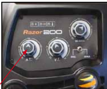
(3) Set the welding current using the amperage control dial.
