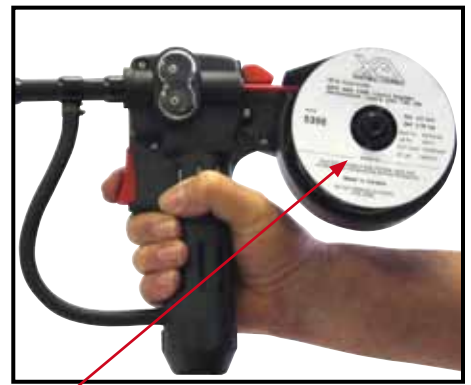
(7) Place a spool of wire onto the Spool holder.
