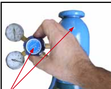
(14) Carefully open the valve of the gas cylinder, set the flow to 8-12 l/min
