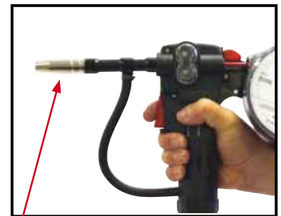
(13) Fit the gas nozzle ready for welding.
