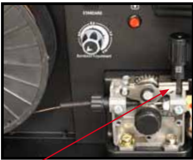
(9) Close down the top roller bracket and clip the pressure arm into place. NOTE: MIG 165 not geared
