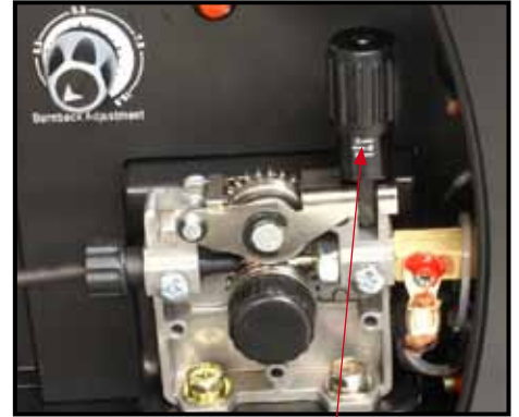
(6) Lock down the top pressure roller and apply a medium amount of pressure using the tension adjustment knob NOTE: MIG 165 not geared
