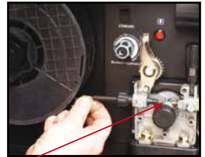
(7) Place aluminium wire onto spool holder. Feed the wire through the inlet guide tube on to the drive roller. NOTE: MIG 165 not geared
