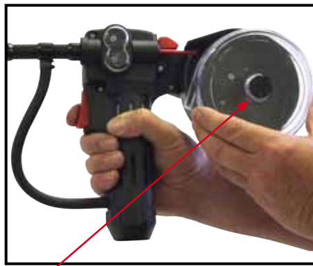
(6) Remove the spool cover by unscrewing the retaining nut and lifting off the cover
