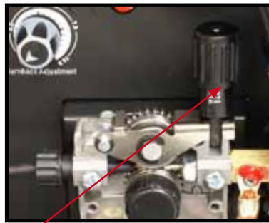
(10) Apply a medium amount of pressure to the drive roller NOTE: MIG 165 not geared
