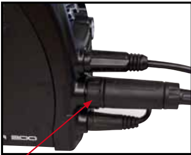
(10) Connect the torch to the machine tighten and secure the torch euro connector to the machine euro connection.
