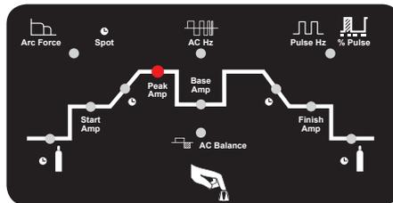
2. Select Peak Amp by pressing the encoder knob to cycle through to illuminate the Peak Amp icon.
