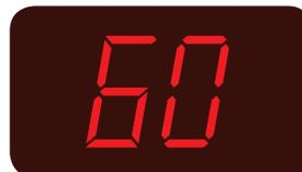
9. Rotate the Adjustment Encoder Knob to set the Pulse Width at 60% - **(Range is 10 - 90%)**
