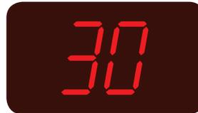
5. Rotate the Encoder Knob to set the Base Amp at 30A - **(Range is 5-180 Amps)**
