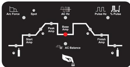
4. Select the Base Amp by pushing the encoder knob to cycle through to illuminate the Base Amp icon.
