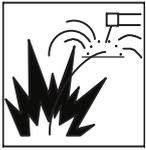
**Fire hazard.** Welding/cutting on closed containers, such as tanks, drums, or pipes, can cause them to explode. Flying sparks from the welding/cutting arc, hot work piece, and hot equipment can cause fires and burns. Accidental contact of electrode to metal objects can cause sparks, explosion, overheating, or fire. Check and be sure the area is safe before doing any welding/cutting.
