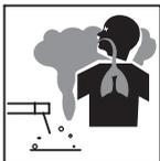
**Fumes and gases are dangerous.** Smoke and gas generated whilst welding or cutting can be harmful to people's health. Welding produces fumes and gases. Breathing these fumes and gases can be hazardous to your health.
