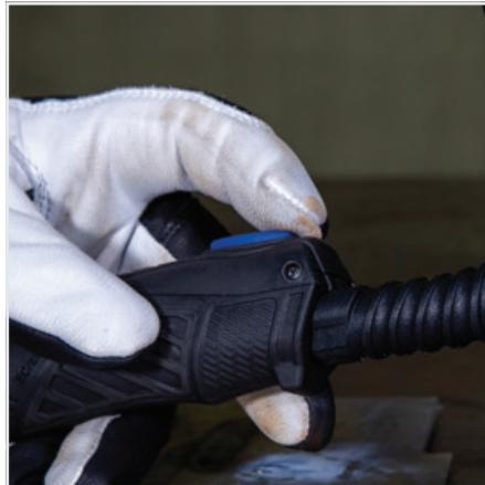
**(2)** Activate the remote control. Press and hold down the torch switch for 5 seconds. The machine will give an audible beep single indicate the remote is activated. Repeat the procedure to de-activate the remote control.
