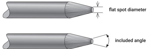
The included angle determines weld bead shape and size. Generally, as the included angle increases, penetration increases and bead width decreases.
