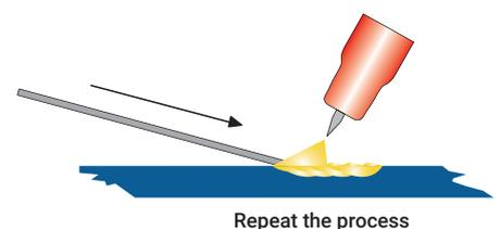
Tungsten is a rare metallic element used for manufacturing TIG welding electrodes. The TIG process relies on tungsten's hardness and high-temperature resistance to carry the welding current to the arc. Tungsten has the highest melting point of any metal, 3,410 degrees Celsius.
