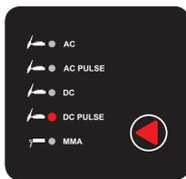
1. Select DC Pulse by pushing selector button to cycle through to illuminate DC Pulse icon.
