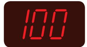
3. Rotate the Encoder Knob to set the Peak Amp at 100A, it will show in the digital display. **(Range is 5-180 Amps)**
