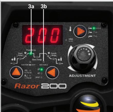
(3a) Push the encoder knob until 'Peak Amp' illuminates, then turn the knob to set the desired amperage.
