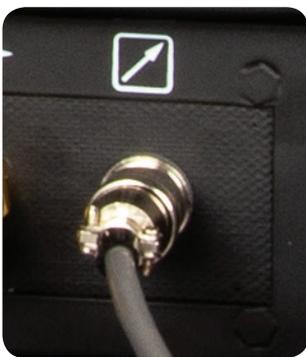
**1.** Connect the remote control 7 pin plug from the Tig Torch switch lead to the 7 pin remote receptacle on the front panel of the machine.
