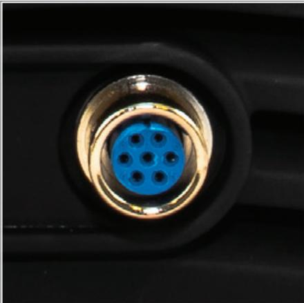
**(1)** Connect the remote control 7 pin plug from the TIG Torch switch lead to the 7 pin remote receptacle on the front panel of the machine.
