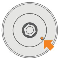
**i** Ensure the wire spool is facing the right direction with the filler wire able to run from the bottom of the spool to the drive rollers.
