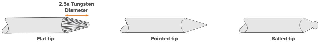
The most common tungsten shape to weld stainless and mild steel with is pointed, which produces a focused and stable arc, and works for all DC applications. To get this pointed shape, you'll need a tungsten grinder or a bench grinder (a diamond wheel is best).
