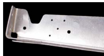
Triple 90° Radius Bend w/ Offset Bend
