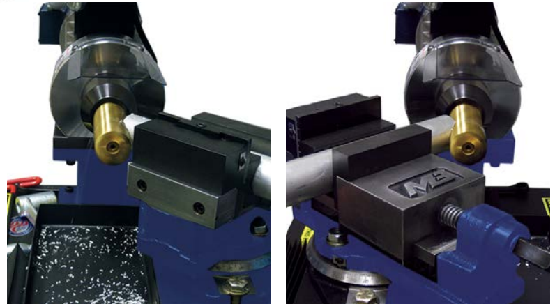
Cluster Joint Created Without Need to Remove from Vise & Reposition Tube
