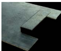
Double Reverse 90° Without Bending Side Legs
