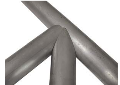
Cluster Joint Created Without Need to Remove from Vise & Reposition Tube
