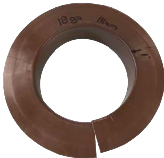
180° Bend Produced Using NEW Stretcher Die # 2700-024
